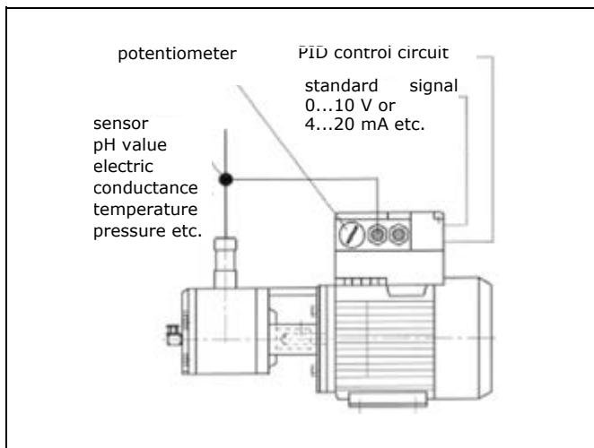
The designs FF and LF with integrated micro-frequency changer permit a rotational speed control of approx. 400 ... 1500 rpm, with larger pumps up to 1000 rpm. The rotational speed can be infinitely set on the potentiometer or fully automatically regulated in the PID control circuit via the standard signal (0... 10 V, 4 ... 20 mA etc.).
