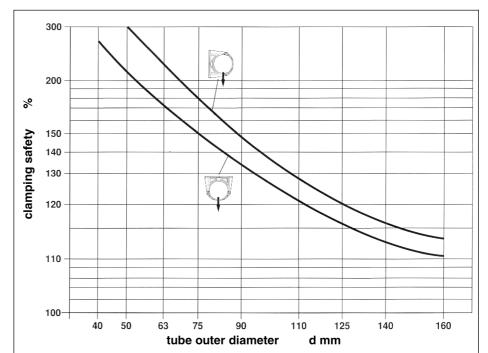
The graph shows the clamping safety (%) against release of the pipe clamp. It refers to the intermediate clamp distances acc. DIN 16928 and same loads, e.g. specific gravity of the media.
